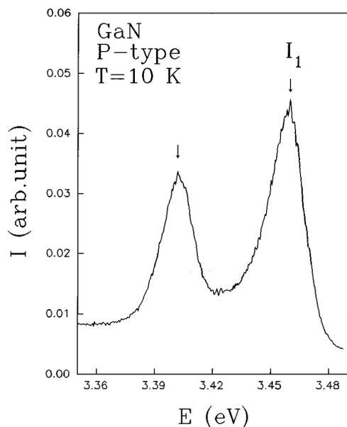
FIG. 1. Continuous-wave (cw) photoluminescence spectrum of an Mg-doped *p*-type GaN measured at  $T=10$  K. The emission line with the peak position at 3.459 eV is due to the recombination of excitons bound to neutral Mg acceptor impurities ( $I_1$ ).
