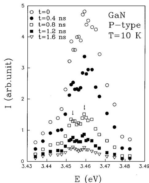
FIG. 2. Low temperature (10 K) time-resolved photoluminescence spectra of the  $I_1$  transition measured at several representative delay times. Two arrows at 3.453 and 3.459 eV in the 0.8 ns spectrum indicate the peak positions of two emission bands resolvable only in spectra of later delay times.
